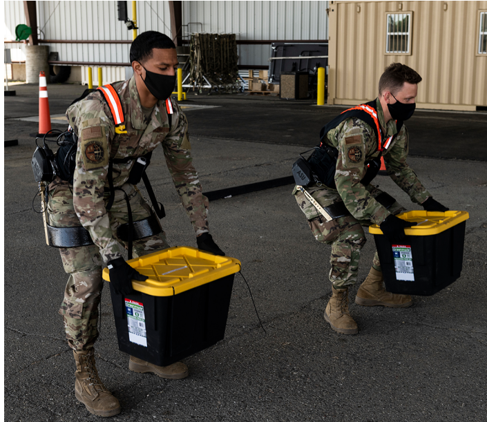
The Aerial Porter Exoskeleton is a piece of equipment designed to reduce strain when lifting various items. Source: U.S. Air Force photo by Senior Airman Cameron Otte
