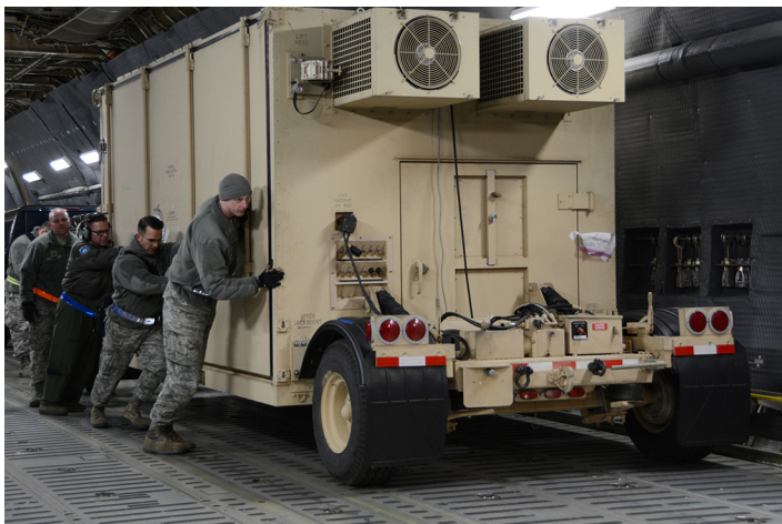
Airmen offload the Hard-sided Expandable Lightweight Air Mobile Shelter from a C-5M Super Galaxy Source: U.S. Air Force photo by Airman 1st Class Hanna Smith
