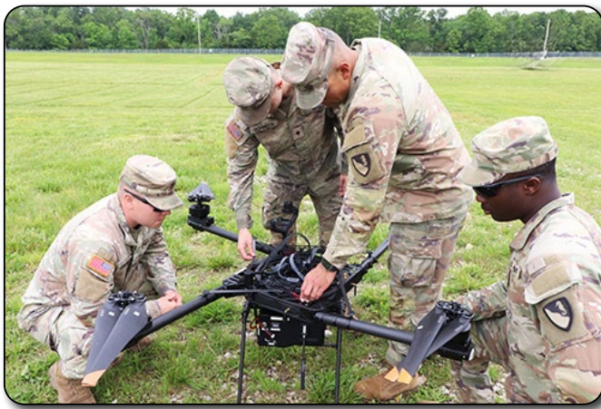
Soldiers operate an Airborne Ground Mines Detection System to identify surface-laid and partially buried mines.
