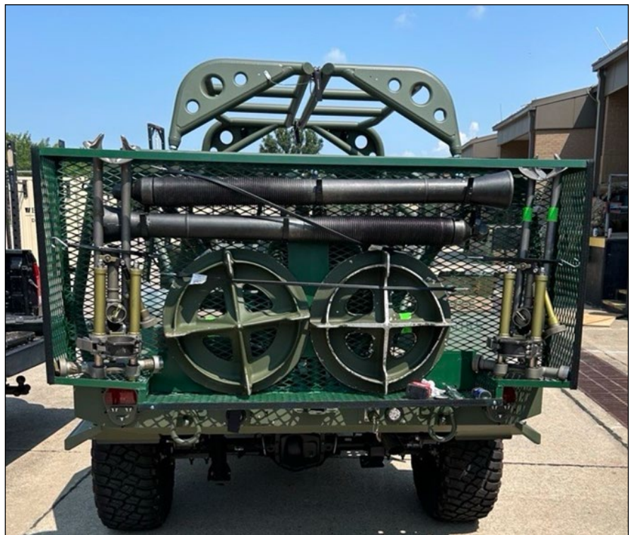
The 2nd Battalion, 502nd Infantry Regiment's mortar platoon fabricated an 81mm mortar-carrying system that attached to the rear of the ISV. (Photo courtesy of author)
