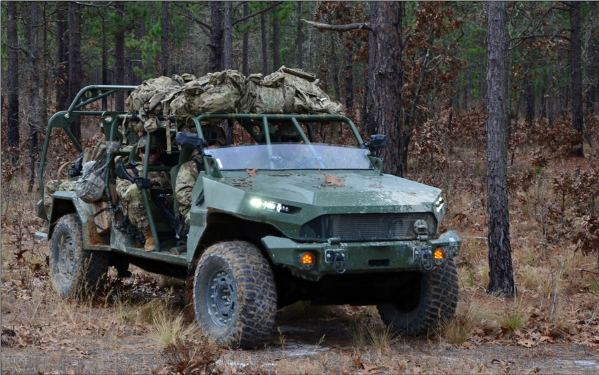
The operational requirements of the Infantry Squad Vehicle include the ability to carry nine Soldiers, a payload of 3,200 pounds, transportable by external sling load by a UH-60 Black Hawk helicopter, internal load/external lift by CH-47 Chinook helicopter, and exceptional mobility over all terrain, allowing infantry brigade combat teams to move with their equipment over difficult terrain. (Photo by Michael J. Malik)
