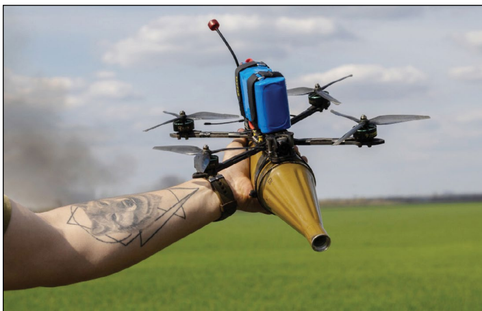
A Ukrainian soldier holds an FPV loitering munition with RPG-7. (Photo courtesy of the Ministry of Defense of Ukraine, armyinform.com.ua)
