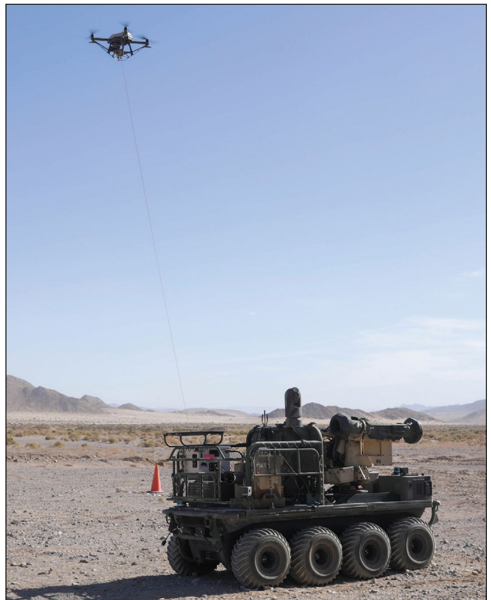
A U.S. Army Origin autonomous weapons system uses a tethered unmanned aircraft system to help Soldiers perform reconnaissance of an area during Project Convergence 22 experimentation on 26 October 2022 at Fort Irwin, CA. (Photo by SPC Jaaron Tolley)
