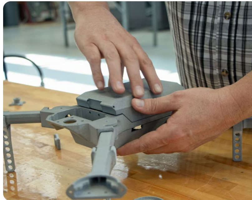
Developed through a proof-of-concept with the 101st Airborne, this drone highlights the potential of 3D printing to quickly create customized tactical equipment. (U.S. Army photo by Kendall Swank)
