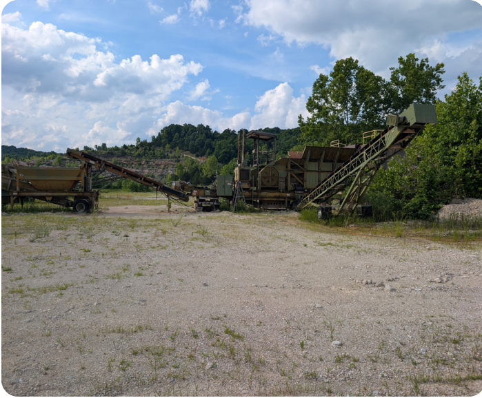
This the equipment is used for quarry AIT and is called the “crusher”
