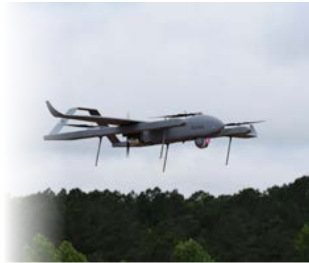
The Aerosonde® Mk. 4.8 Hybrid Quad UAS at Redstone Arsenal, Alabama. Courtesy photo: Program Executive Office, Aviation.
