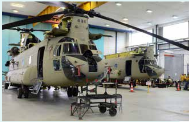
U.S. Army Soldiers conduct 400 hours phase maintenance on a CH-47 Chinook. U.S. Army photo by Charles Rosemond.
