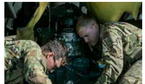
U.S. Army aircraft maintainers work on the combining transmission box of a CH-47 Chinook for a 160-hour phase maintenance inspection during a multinational training exercise. U.S. Army photo by SGT Jason Greaves.
