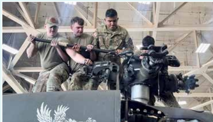
Company B, 602D Soldiers conducting a 960-hour phase maintenance inspection on a UH-60L in June 2024. Photo courtesy of CW3 Tim Clafin.
