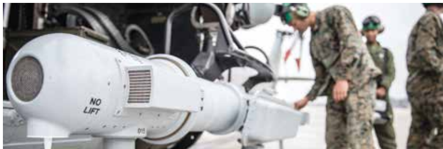
A UH-1Y Venom is staged on the flightline with an AN/ALQ-231(V)3, which enhances the airborne electronic warfare capability for fixed- and rotary-wing aircraft. U.S. Marine Corps photo by Sgt Samuel Ruiz.
