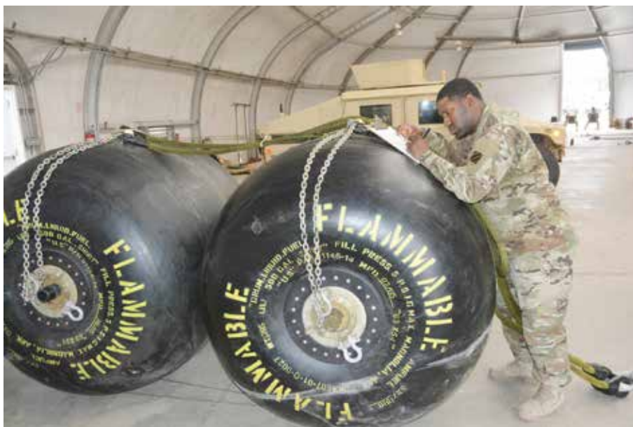
SPC Prentis Ficklin inspects fuel blivets to ensure they are ready to be sling loaded. U.S. Army photo by SPC Rochelle Krueger.
