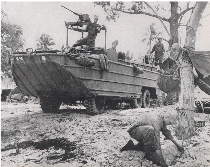
Soldiers of 1st Signal Troop emplacing wire using a DUKW amphibious vehicle at Los Negros Island. (Photo from Signal Historical Collection)
