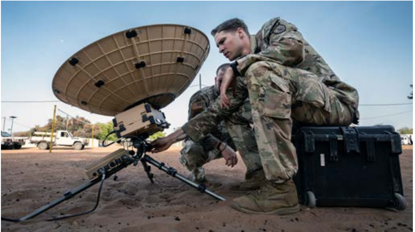
SSG Devin Sasser, network communications systems specialist, Maneuver Combat Advisor Team 2310, 2nd Security Force Assistance Brigade, config-ures a microwave satellite terminal to increase tactical communication to support exercise African Lion 2024 in Dodji, Senegal, May 27, 2024. (Photo by SFC Nicholas J. De La Pena)
