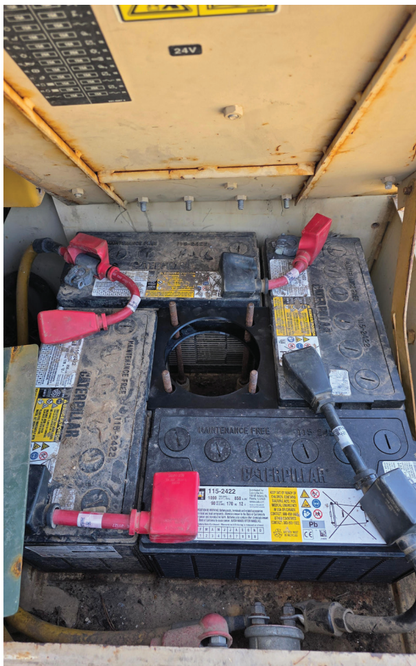
Figure 1: D7 Dozer batteries with retainer missing (Photo by 1LT John Douglas)
