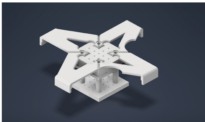
Figure 3. Side view of CAD rendering of battery retainer created by the Innovations Cell. (Photo by 1LT John Douglas)
