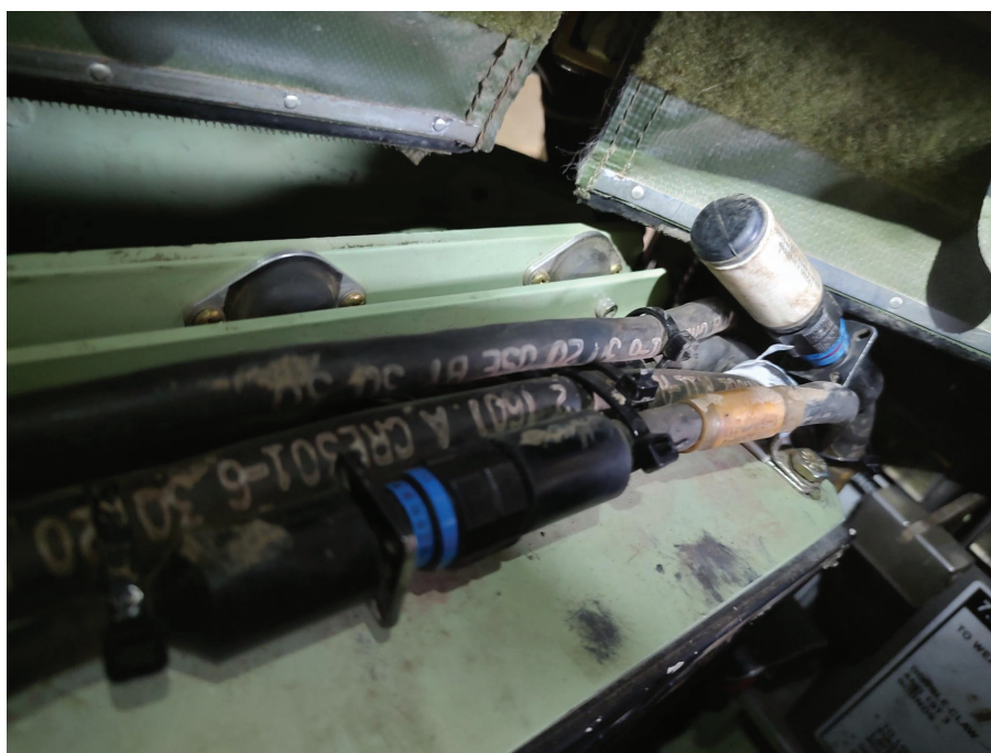
Figure 5. Image of CAN bus cables without bracket installed. (Image by SFC Donald Fadel)
