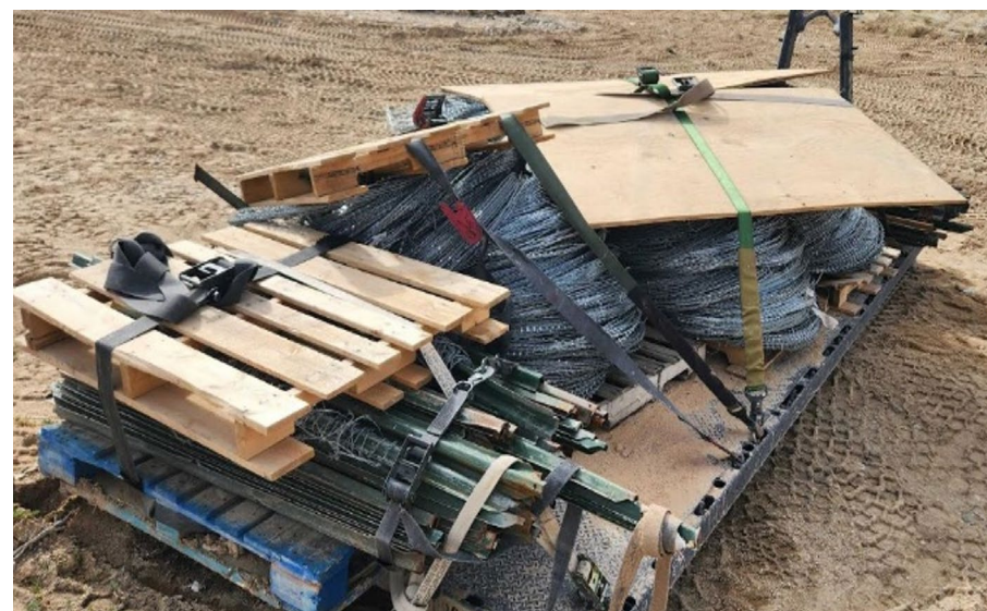
Figure 1. Poorly built CCL loaded with concertina wire, pickets, and barbed wire. Note the Concertina Wire falling over and randomly placed ratchet straps. (U.S. Army photo by CPT Olivia Schretzman and MAJ William Longwell)
