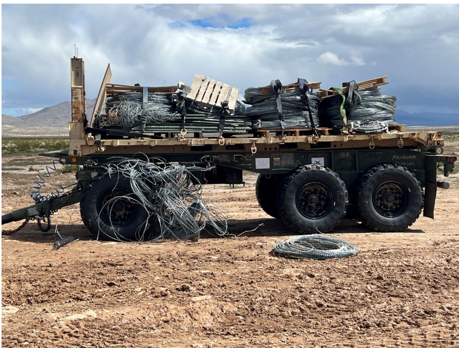
Figure 2. Consequences of a poorly built CCL, Concertina Wire falling off and into an axle. (U.S. Army photo by CPT Olivia Schretzman and MAJ William Longwell)
