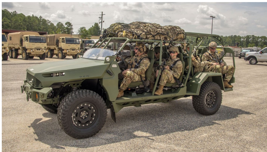
Figure 3. Paratroopers assigned to the Airborne and Special Operations Test Directorate prepare to depart for a 50-kilometer road test in a fully loaded Infantry Squad Vehicle (ISV). (U.S. Army photo by Michael Zigmond)
