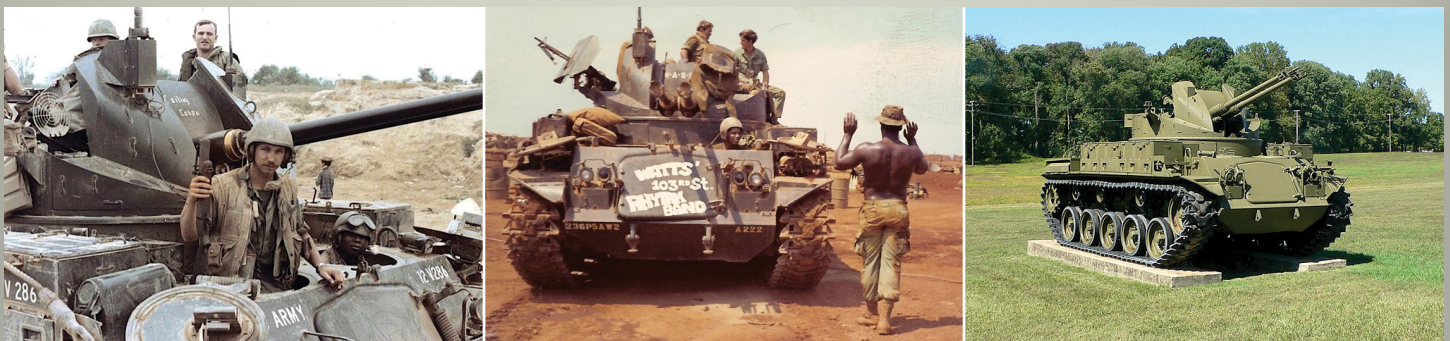
The M42 40 mm Self-Propelled Anti-Aircraft Gun, or “Duster,” is an American armored light air-defense gun built for the United States Army from 1952 until December 1959, in service until 1988. (Photo credits: Left, Mark Pellegrini, U.S. Army Ordnance Museum [Aberdeen Proving Ground, MD] Creative Commons CC-BY-SA-2.5; Middle: the Army Historical Foundation; Right: Bill Maloney, Pennsylvania Military Museum)
