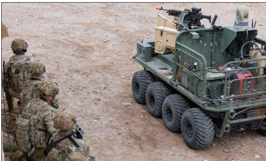
A U.S. Army unmanned, eight-wheeled, all-electric, all-terrain transport vehicle armed with the R600 autonomous weapon system provides support to dismounted Soldiers as part of a human integration experiment. (Photo by SPC Samarion Hicks)
